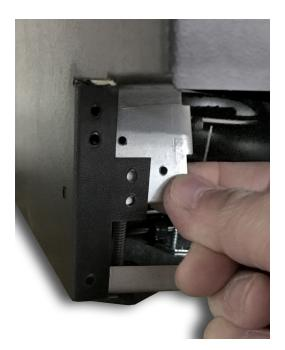
3. Use two adjusting screws to install bracket; tighten screws with provided Allen wrench.
