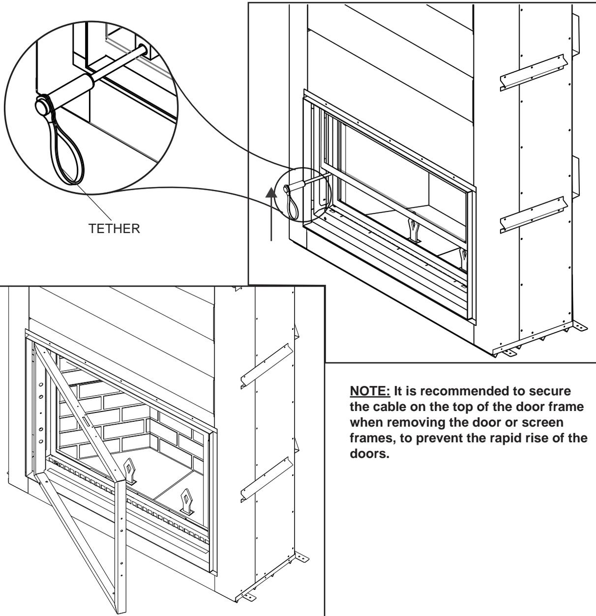
**NOTE:** It is recommended to secure the cable on the top of the door frame when removing the door or screen frames, to prevent the rapid rise of the doors.
