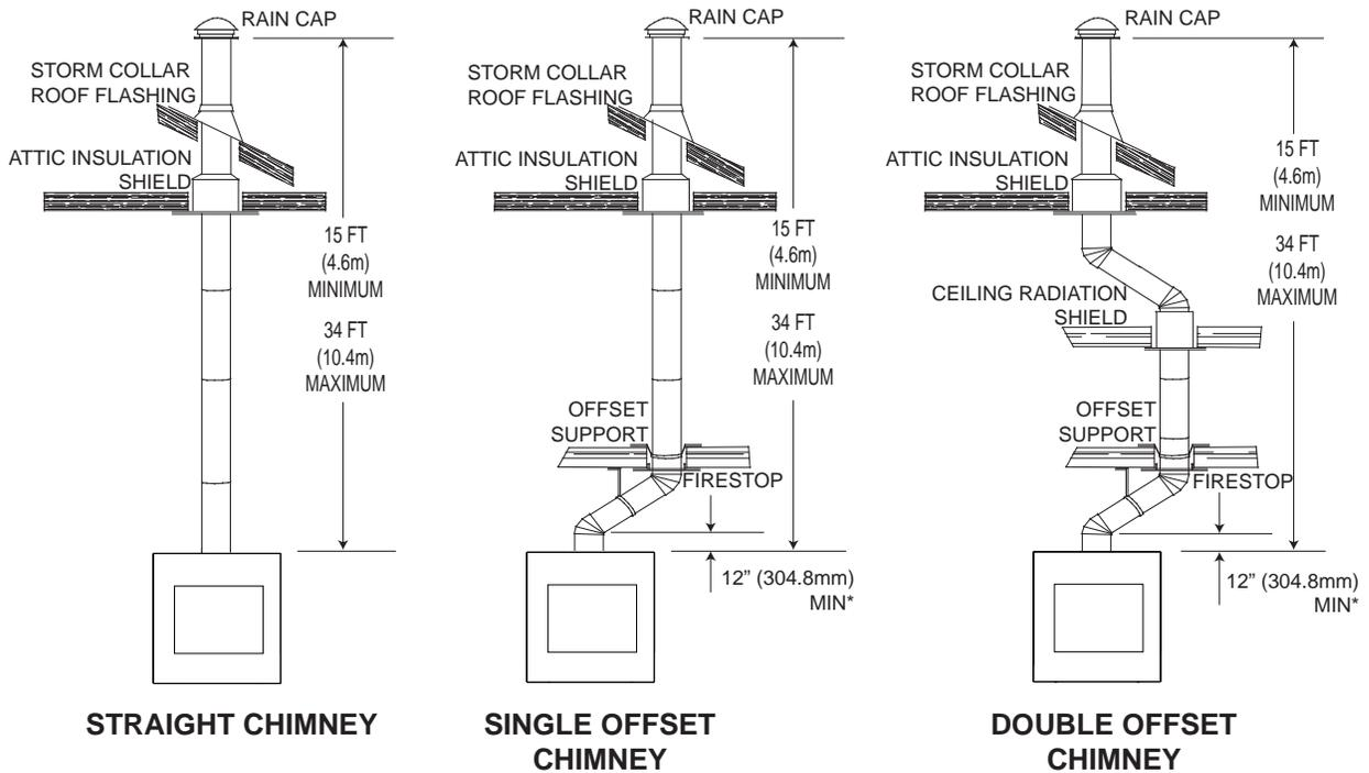
\* The first flue offset closest to the top of the appliance must be a minimum distance of 12" (304.8mm) from the top of the appliance.
