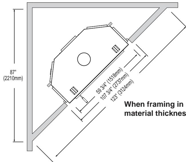
**When framing in unit, allow for finishing material thickness.**
