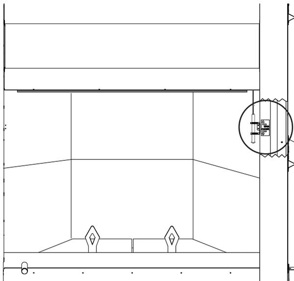
To close the damper, pull the damper control rod down and push it to the right.
