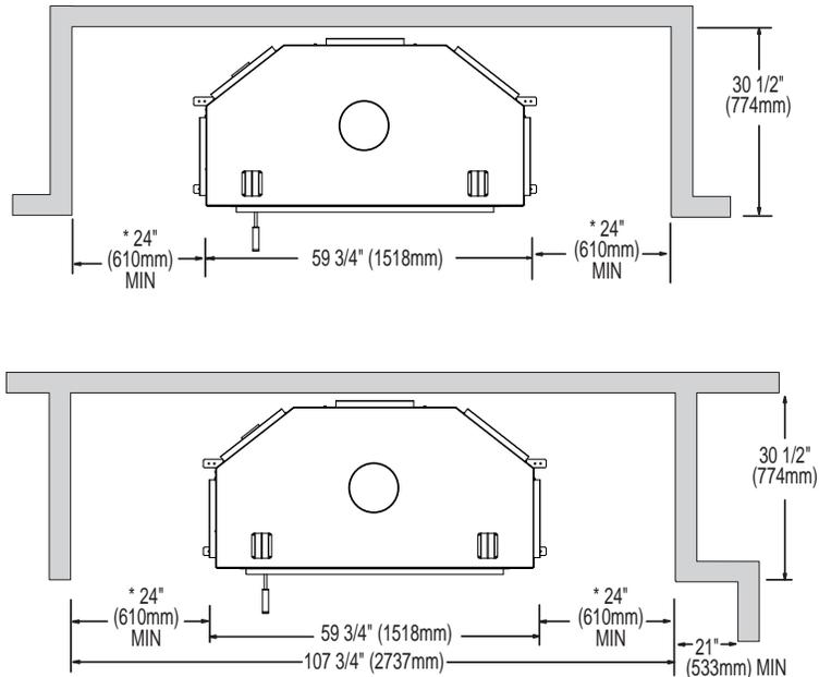
**\* It is recommended to leave a min of 24" (610mm) of clearance to the sides of the appliance to facilitate servicing either the guillotine door or the screen door operating systems; access to this space will need to be considered.**
