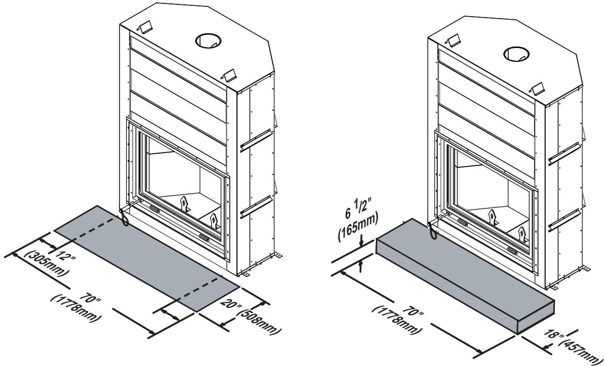
An acceptable 61½" (1562mm) x 20" (508mm) non-combustible (ie: brick, stone or ceramic tile) hearth extension must be installed. Hearth must extend 20" (508mm) in front of the faceplate when it is not elevated (see local building codes). Hearth must extend a minimum of 12" (305mm) to both sides of the appliance [70" (1778mm)].
