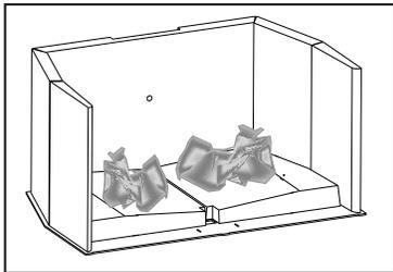
**A.** To start, a brisk fire is required. Roll up some newspaper (loosely crumpled), light it and place it near the appliance flue until the chimney begins to draw.
