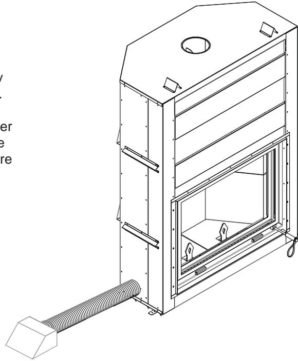
The duct inlet must be located so they can not be blocked (i.e. snowdrifts). 12" (305mm) above grade is recommended. Make a 4 ½" (114mm) inch hole to suit in an outside wall of the house. From outside, place the fresh air hood into the hole, open side down. Seal with caulking and secure.
