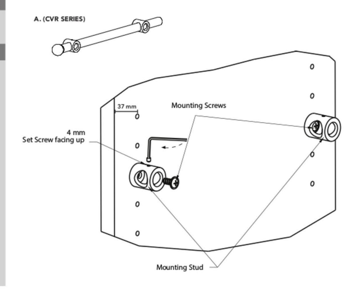
These units can be unassembled and flipped, see back for details.
