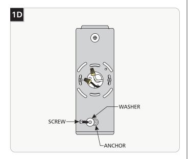
Slide a #8 screw through a washer and screw it into an anchor. Repeat for the other anchor to secure the mounting plate to the wall.
