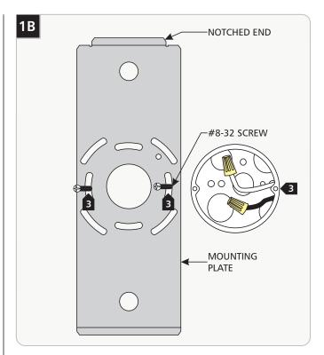
Attach the mounting plate to the electrical box using the two #8-32 screws provided. Make sure the notched end of the mounting plate is at the top.
