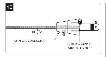
7 Feed and push the coaxial cable into the conical connector. The coaxial cable will come to a stop point after being inserted 3/4" into the conical connector.
