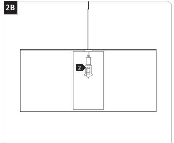
Use MAX 50 Watt, Bi-Pin Halogen Lamp.
