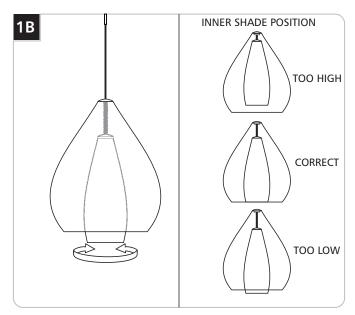
2 The inner shade position is set at the factory, but may shift during shipment and installation. If necessary, spin the inner shade to move it up or down.
