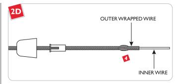
**1** Slide the outer wrapped wire back to expose the inner wire.
