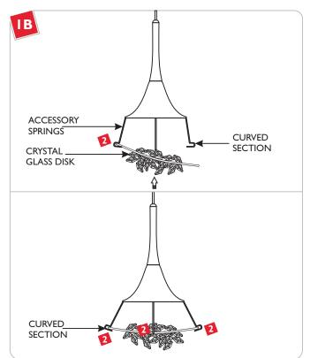
Orient the recessed section of the crystal glass disk toward the lamp. Place edge of the crystal disk into curved section of accessory springs.
