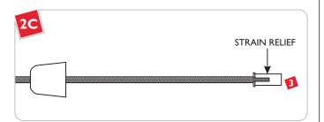
Insert the coaxial cable through the flared end of the strain relief.
