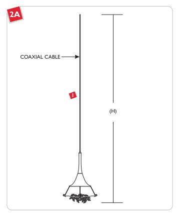
Cut the coaxial cable to the desired length with a sharp cutter. The overall fixture height (H) is measured from bottom of the crystal glass disk to end of the coaxial cable.
