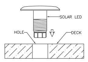
3.) Secure the Solar LED Light to the deck using the locking ring.
