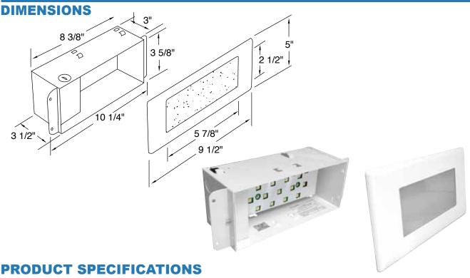
Description: LED step light, suitable for use on stairs, wall bases, or any indoor or outdoor applications requiring safe illumination in dark areas. Stamped painted steel housing, powder coated. (3) 1/2" knockouts are provided.
