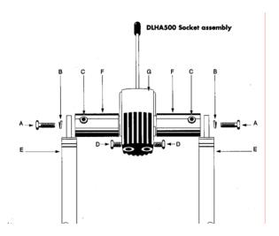
To install or remove screw "A", the set screw "C" must be loosened (allen key not provided). Screw "A" will not loosen or tighten without first loosening set screw "C". If you try to tighten screw "A" without loosening set screw "C" you will break arm "F" from base of socket "G". Breakage of arm "F" is not covered under warranty.
