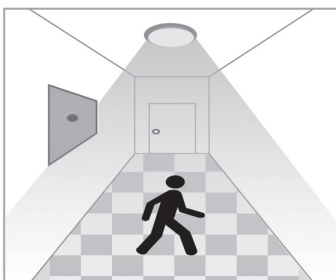
When motion is detected, the sensor will switch ON the light to 100% brightness.
