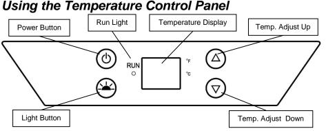
Use the up and down buttons to adjust the temperature. The temperature displayed can be in Fahrenheit or Celsius. This kegerator has a temperature range from 32°F to 60°F.
