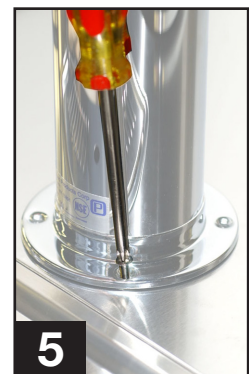
Thread beer line connector to draft arm and secure draft arm to cabinet with rubber gasket under the draft arm.
