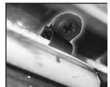
P-Clip keeps cord in-place (prevents cord damage).
