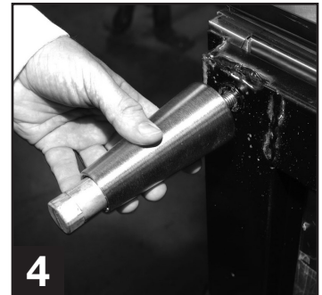
4 Thread leg into cabinet bottom frame rail.
