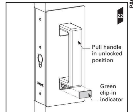
**23.** If installing a handle with snib both sides, fit the clip-in indicators to both sides.
