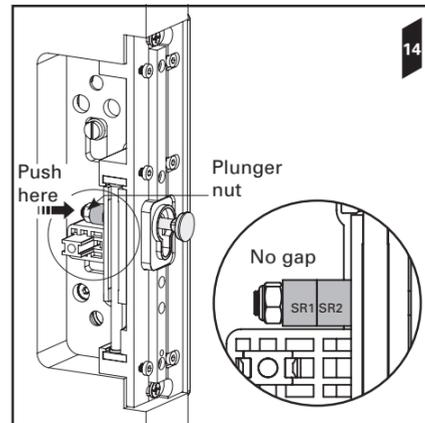
**15.** Place the **small** end of the second spanner across the flats under the head of the *plunger*. Keep the spanner restraining the plunger nut **stationary** while turning the second spanner **clockwise**. Continue to turn the spanner until there is no longer a gap between the spanner and the shroud face.
