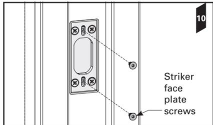
**11.** Position the striker face plate in the centre of the striker body - this may need to be adjusted in the steps following. Insert the striker face plate screws and loosely tighten.
