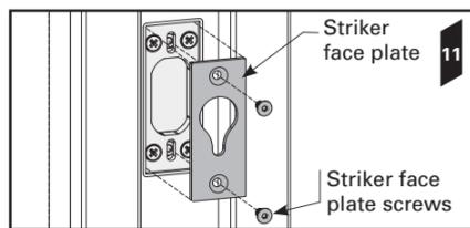
**12.** Close the door. When the striker is fitted correctly the magnet will draw the plunger forward. If this does not happen the striker is misaligned with the plunger (see below). If the alignment is correct, tighten the screws and skip to **Step 14**; otherwise continue to **Step 13**.
