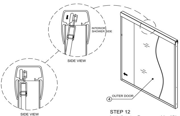
Install outer Door panel by lifting up & into Top track (1) ( Do not lift by towel bar, be careful not to bump panel against metal track.)
