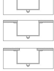
The instructions that follow are for installing a Kingston Brass undermount stainless steel sink in a solid surface countertop only. Minimum thickness of the actual countertop material is one half-inch. In addition, a one-inch build up around the sink is preferred. Kingston Brass recommends that undermount sinks and routering of your solid surface material should be Installed by a professional installer for best results.
