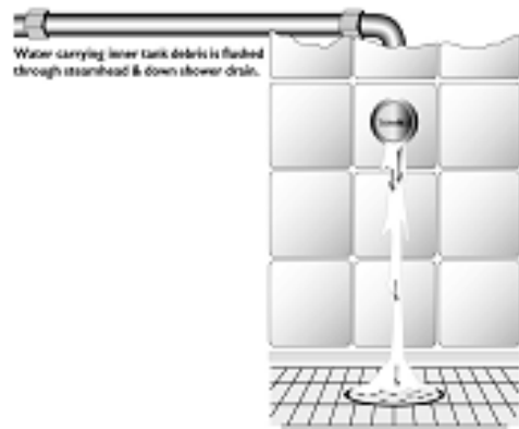
Figure 4: Tank maintenance - power cleaning the tank.
