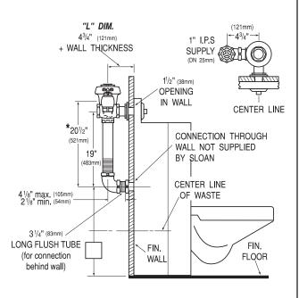
\*For Solenoid Operated Flushometers (ES and ESM variations) the Water Supply Rough-in dimension is 16" (406mm).
