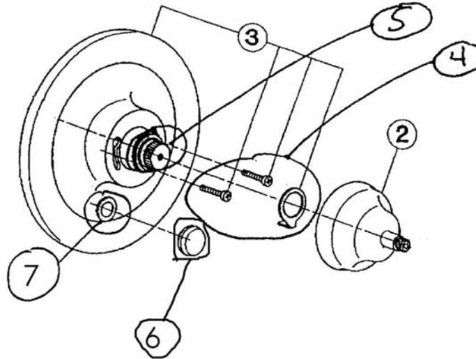
MOUNTING SCREWS+CAM+DIVERTER ASSEMBLY
