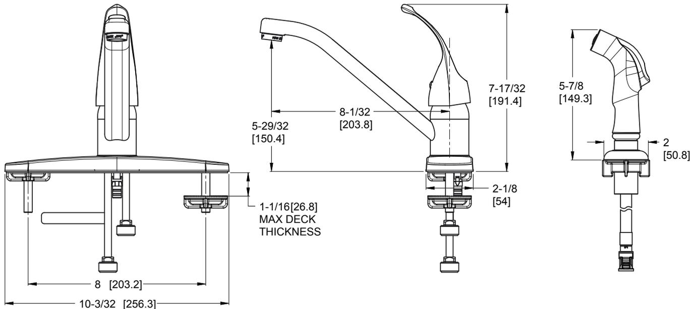
Ø1-3/8 Min to Ø1-1/2 Max. Deck Hole Openings
