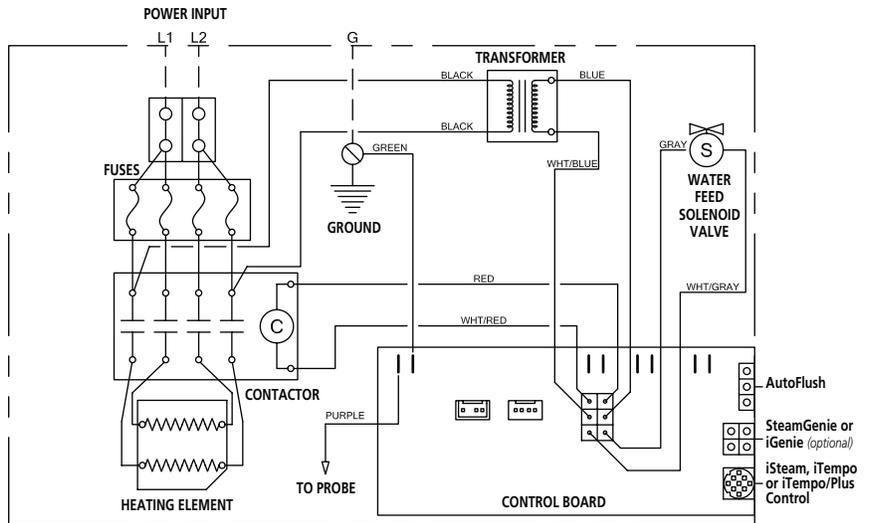
**THREE PHASE 208/240 VOLT WIRING DIAGRAM**
