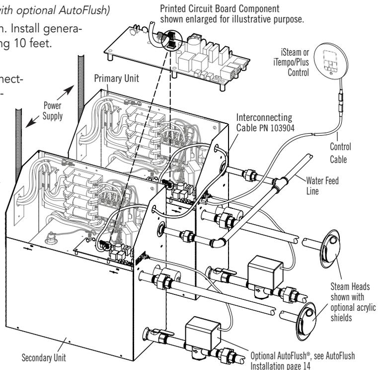
**NOTE:** The secondary unit will de-energize when the steam room reaches steambathing temperature resulting in a more gentle and energy efficient operation.
