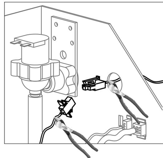
1. Remove the connector from the "C" location in the jacket. Cut off the connector where shown and strip back the wires approx 0.375"
