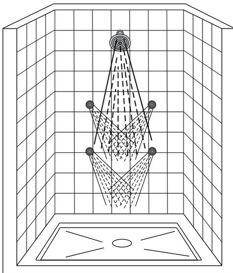
This design utilizes a showerhead and multiple body sprays to ensure complete water coverage.
