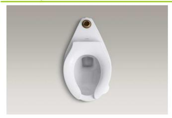
The elongated toilet bowl shall be made of vitreous china. Bowl shall be 28-1/4" (718 mm) in length, 14-7/8" (378 mm) in width, and 15" (381 mm) in height. Bowl shall be 10" (254 mm) or 12" (305 mm) rough-in with 1-1/2" top spud. Bowl shall be 1.28 gpf (4.8 lpf) or 1.6 gpf (6.0 lpf) depending on flushometer specified. Bowl shall have 11" (279 mm) by 9" (229 mm) water area. Bowl shall have 2-1/4" (57 mm) passageway. Bowl shall have bedpan lugs (-L).
