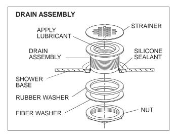
Remove the stainless steel strainer from the drain assembly. Disassemble the locknut and two gaskets from the back of the drain assembly. Apply a 1/4" bead of caulking (silicone) to the drain hole and insert the drain assembly. Replace the rubber washer, fiber washer, and lock nut in that order. Hand tighten the locknut. Remove excess sealant from finished side. (See illustration).
