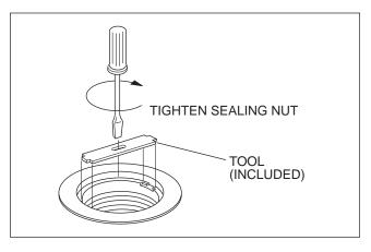
With a large screwdriver and the tool included with the drain, tighten the inside compression nut to seal the drain pipe connection. Replace the strainer and tape over the drain hole to prevent finishing material from entering drain.
