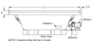
Letter Description **English** Metric 72" Outer Length 1829 mm W Outer Width 42" 1067 mm Overall Height\*\* 24" 610 mm Overflow Height 17" 432 mm Α В Long Edge to Drain Center 10 1/4" 260 mm С Short Edge to Drain Center 36" 914 mm D 8 1/2" Drain Shoe Length 216 mm Ε Deck Height\*\* 4" 102 mm F Deck Width\* 3 1/2" 89 mm G 12" H x 18" L Service Access Dimensions 305 mm x 457 mm 18 ½" x 4" Floor Cut-out for Drain 470 mm x 102 mm
