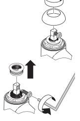
Replace the high temperature limit stop so that the pin on the cartridge is in the desired slot on the limit stop. *Note:* the temperatures given in the diagram assume a water heater temperature of 140° F, a cold water temperature of 50° F, and a water pressure of 45 PSI. Your high temperature may vary.
