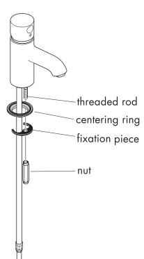
Install the pop-up drain. Install the pull rod and connect to the drain assembly.
