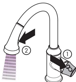
Press the diverter to obtain the spray mode. The diverter will reset to stream mode when the water is turned off.
