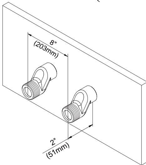
2. Wrap pipe sealant tape around threads of supply pipes, then thread on the offset adaptors onto the pipe. Adjust the orientation of the offset fitting to 8" center to center. Tighten securely.
