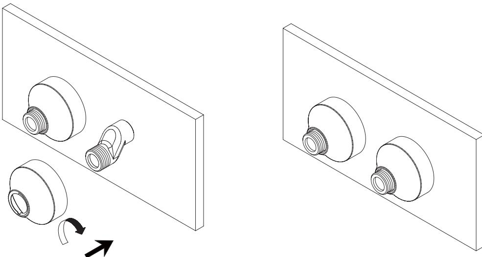
**3. Thread on escutcheon to the offset adapter.**
