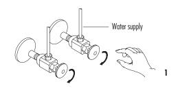
Remove rubber washer, metal washer, lock nut and spout connector from the spout shank. Position the spout in the faucet hole of the sink. Slide the rubber and metal washers up the shank and secure spout with the lock nut. Wrap end of mounting shank with pipe tape and reattach spout connector. Do not overtighten.
