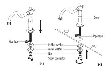
Remove lock nut, rubber washer and metal washer from hot valve body. Wrap male threaded end of flexible spout connector hose, and install in bottom of valve body. Insert valve body through the correct faucet hole, replace rubber and metal washers, and secure with lock nut.
