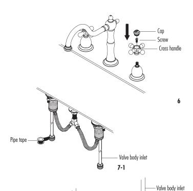
After attaching supply lines, remove aerator and turn on hot and cold water for 1 minute to flush the lines. Replace aerator. Check for leaks.
