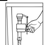
Turn on water supply. Adjust water to desired level by squeezing water level adjustment clip and moving FLOAT CUP up or down along stainless steel link.
