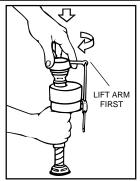
• Replace TOP by engaging lugs and rotating 1/8 turn clockwise. MAKE CERTAIN TIP IS TURNED TO THE LOCKED POSITION.
