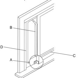
A. Window locking bracket B. Window sash sealing strip C. Inner window D. Outer window
