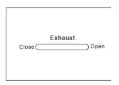
The Exhaust Control allows the air conditioner to either circulate inside air (Closed) or exhaust air to the outside (Open.) The Closed position is used when maximum cooling is desired. The Open position removes stale air from the room and exhausts it to the outside.
