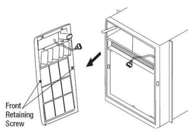
$\underline{\underline{NOTE:}}$  Be careful not to push or pull the louvers when removing the front panel.
