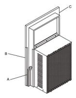
A. Side channel sealing strip B. Side channel C. Window panel frame
