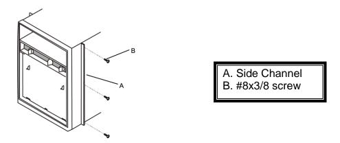
4. Slide the plastic window panel into the window panel frame with the smooth side facing the flat edges of the panel frame. Once the plastic window panel is in place, slide the panel frame assembly down into the side channels until the bottom of the plastic panel rests inside the groove on top of the air conditioner.
