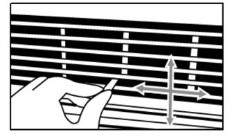
The 4-way air directional louvers allow you to direct the air flow Up, Down, Left, and Right throughout the room as needed. To adjust the air directional louvers side to side use the center handles as you move side to side. To pivot the louvers, press with your fingers until the desired airflow direction is obtained.
