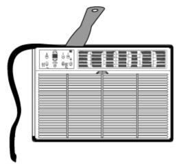
2. Locate the 4 (four) trim kit components that were packaged with your installation kit. Snap the pieces together as shown in the image below.
