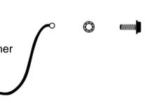
2. As needed, use a drill and  $\frac{1}{8}$ " bit to drill a hole for the grounding screw. The hole needs to be approximately 1" from the bottom and 3" from the front edge of the wall sleeve on the left side.
