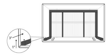
3. Attach one end of ground wire using 1 (one) Toothed Washer and 1 (one) Grounding Screw.
