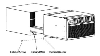
3. Gently slide the air conditioner cabinet into the Wall Sleeve. With the cabinet screw hole still exposed, attach the ground wire to the cabinet using the cabinet screw making sure that the Toothed Grounding Screw Washer is pressed against the cabinet.
