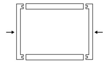
3. Pull the power cord through the Trim Kit frame and then slide the Trim Kit Frame over the unit until it is flush with the wall.
