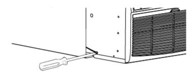
4. Slide air conditioner completely to the rear of the wall sleeve unit ensuring that all seals and foam support blocks create snug fit for the unit. Please be sure that the ground wire does not become entangled when the unit is pushed back into the wall sleeve.
