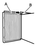
6. Then insert the bottom of the side curtain housing into the bottom channel on the air conditioner as shown below:
