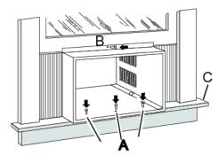
A. #10 x ½" Phillips Screws B. #10 x ¾" Flat Screws C. Window Sill
