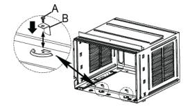
A. #10 x ¾" Phillips Screw B. Safety Locks (Only for Vinyl Windows) Check that the air conditioner cabinet is tilted back about 1 <sup>1</sup>/<sub>8</sub>" to 1 <sup>1</sup>/<sub>2</sub>", which should be about 3-4 degrees downward to the outside. After proper installation, condensation should not drain from the overflow drain hole during normal use, correct slope or otherwise.
