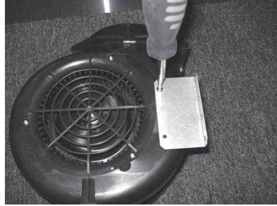
7. Attach blower brackets to blower with (4) 10x3/16" screws. (2) screws for each bracket.
