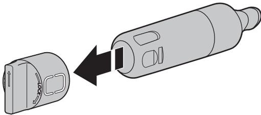
5. Install the water filter cap onto the new filter. Be sure to align the arrows so the grooves in filter align with ribs in filter cap.
