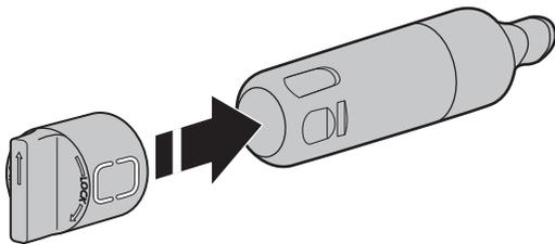
6. Insert the filter into the housing.
