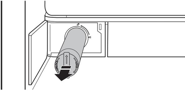
4. Remove the water filter cap from the water filter being replaced.
