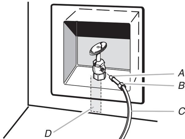
A. Sleeve B. Nut C. Copper tubing (to refrigerator)
