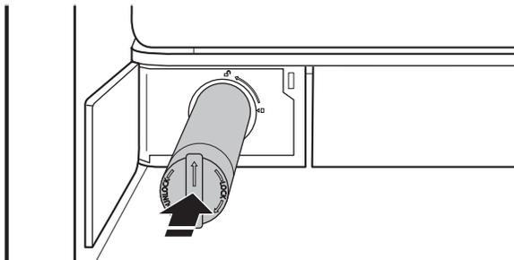
7. Twist the water filter and turn 90° clockwise until it locks into place and the arrows are aligned.
