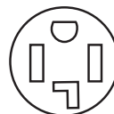
4-wire receptacle (14-30R)
