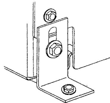
5. Adjust the anti-tip bracket so that it rests securely on the floor. **TIGHTEN THE SCREW COMPLETELY.**
