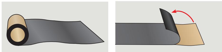
**ENGLISH:** To ensure waterproofing, skylight curbs shall be completely wrapped in VELUX adhesive skylight underlayment as indicated. Underlayment must be applied before installing the flashing. Remove existing roofing underlayment around the rough opening as shown.
