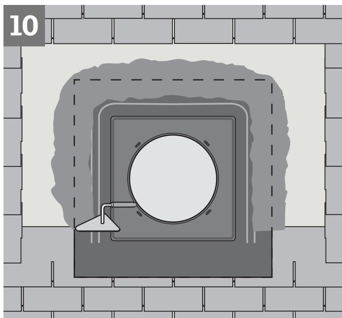
**ENGLISH:** Apply sealant as shown and seal all fasteners.
