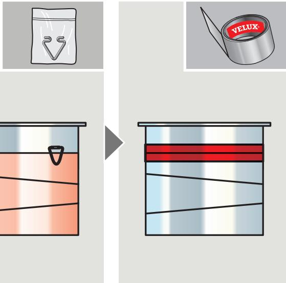
**ENGLISH:** Attach the upper elbow to the top collar. Secure joints with tunnel clips and tape provided.
