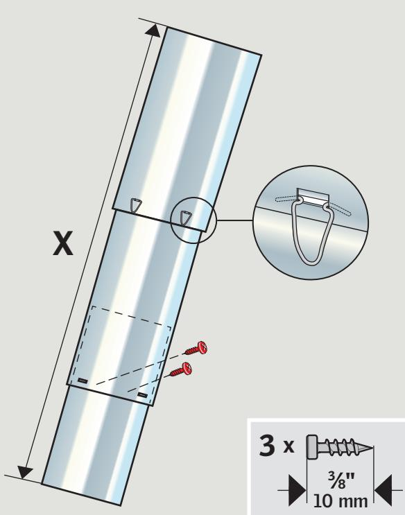
**ENGLISH:** With more tunnel sections, assemble the upper sections with the tunnel clips provided and reduce the length of the tunnel assembly by increasing overlap at the bottom. Secure the joint with three of the  $\frac{3}{8}$ " (10 mm) screws.
