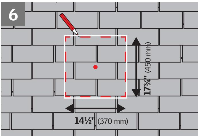
**ENGLISH:** Locate the nail indicating the center of the sun tunnel on the roof and mark rough opening.
