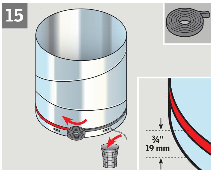
**ENGLISH:** Attach pile gasket to lower elbow as shown.
