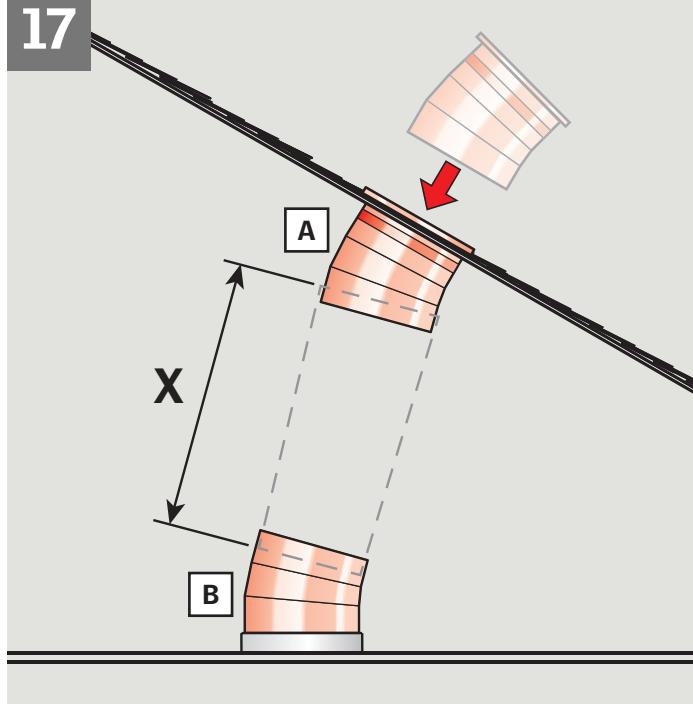
**ENGLISH:** Adjust the angle of both elbows so that they point directly against each other **A**, **B**. Elbows can be damaged if excess force is applied.
