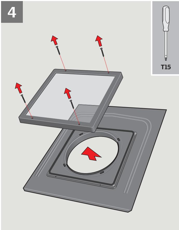
**ENGLISH:** Unscrew and remove lens from flashing.
