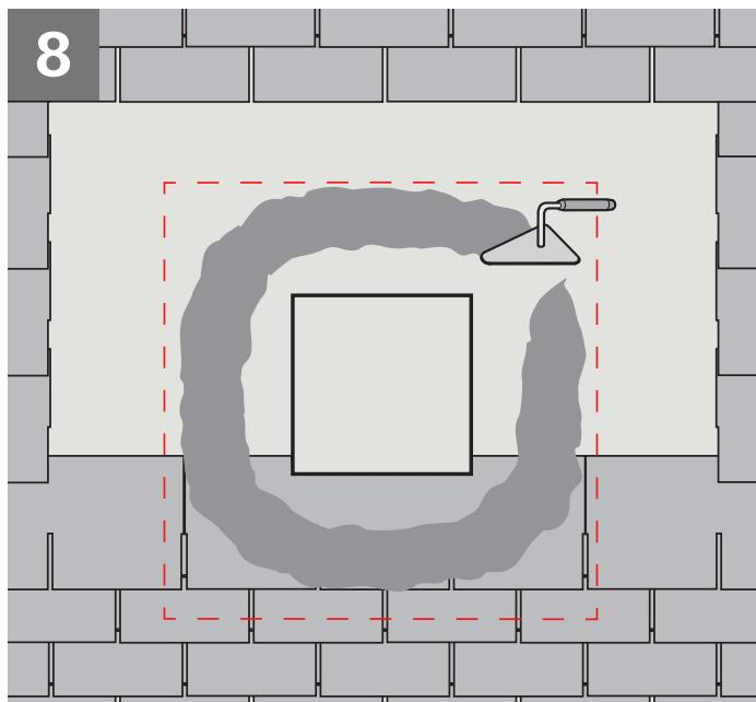
**ENGLISH:** Remove the roofing material around the upper half of the rough opening as indicated and apply mastic around rough opening as shown.
