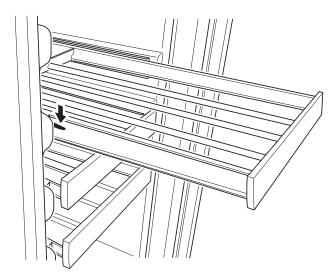
Press the left rack release lever down. At the same time, lift the matching right rack release lever up.
