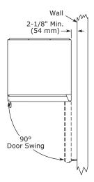
Units have a zero clearance for the door to open  $90^{\circ}$ , when installed adjacent to cabinets.
