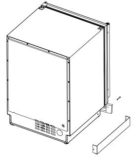
3. Align front hole wit hole in shell accessory, hole in base, and hole in grille. Tighten screw.
