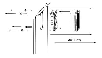
14. Remove and replace fan. Take special care to properly route fan wire.
