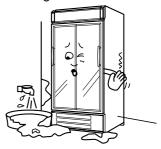
Ambient temperature should be below 85°F. Warmer temperature will cause problems with cooling efficiency.
