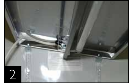
Shelf clips are installed with the front clip lower than the rear clip. This will allow the shelf to tilt forward.
