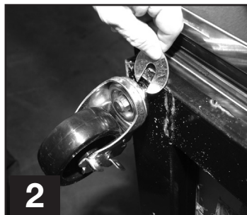
2 For leveling, insert the shim between the castor and frame rail.
