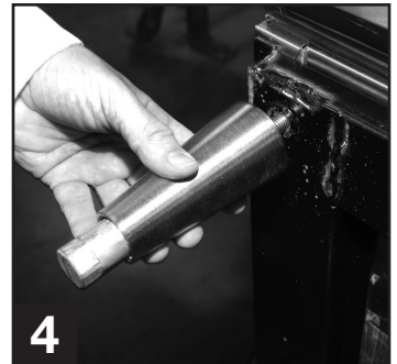
4 Thread leg into cabinet bottom frame rail.
