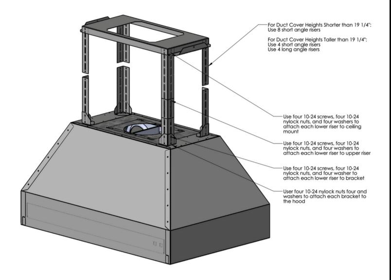
**IMPORTANT:** For ceilings higher than 10', a "chase" or soffit must be constructed prior to hood installation, in order to secure the included duct cover.
