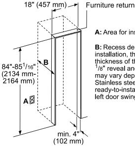
A: Area for installation of power connection.
