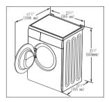
The dimensions shown are for the recommended spacing. Custom dercounter installation
