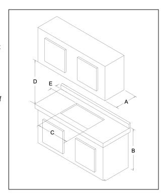
**NOTE:** Do not install closer than 1/2 in. (12 mm) from any adjacent surface.
