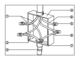
**NOTE:** Do not connect the bare ground wire to the neutral (white) wire in the junction box.
